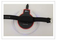
Blue LED lights on the charger will slowly flash on and off repeatedly to confirm the wristband is charging.
